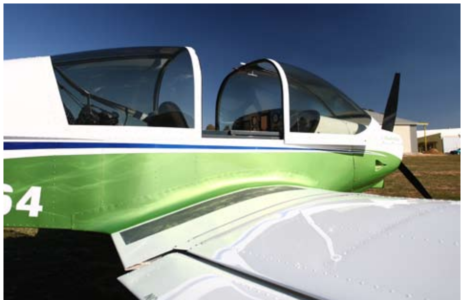
ROOMY WITH A VIEW Access to the roomy two-seat cockpit (left) is via the large forward sliding canopy (right).
