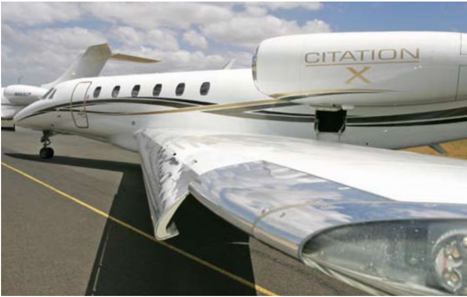
GOT IT RIGHT The wing is not only highly swept, it is very clean.
