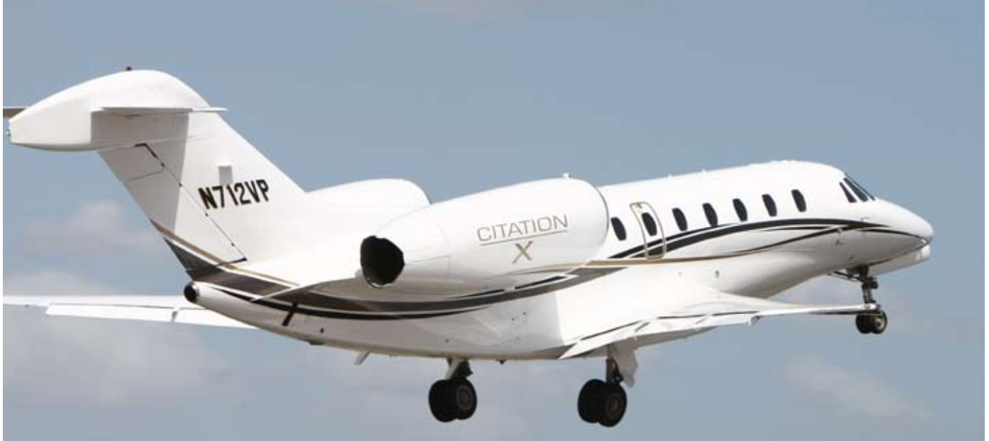
DANGLING DUNLOPS The X features dual wheeled main and nose landing gear.
